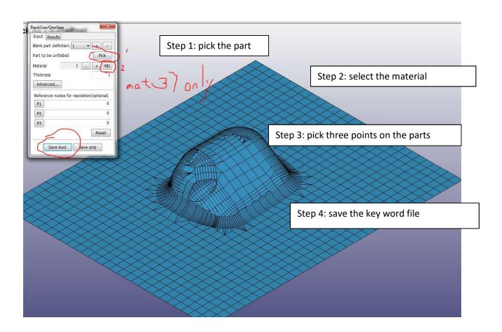
Write out a keep word file. For example test.k
